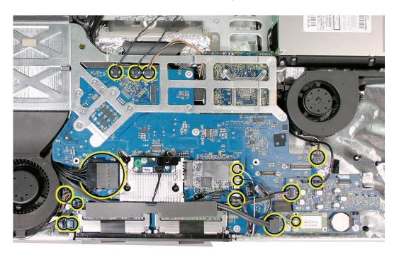
Remove the thirteen screws from the logic board. Note that the machine screw location has an arrow designation stamped onto the metal backer plate.
